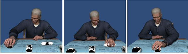
**Figure 5:** Examples of grasping objects with various shapes. Our system determines hand orientations and finger poses based on object shapes and collision detections.
